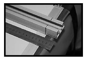
C) Cut all 4 ends! Use a hack saw or other tool of choice for cutting through aluminum.
