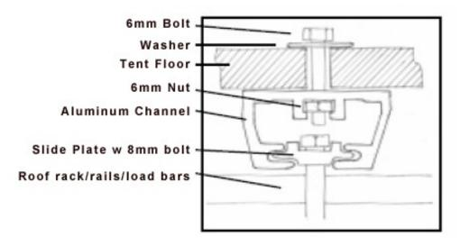
**B)** Slide 2 6mm nuts into each channel.
